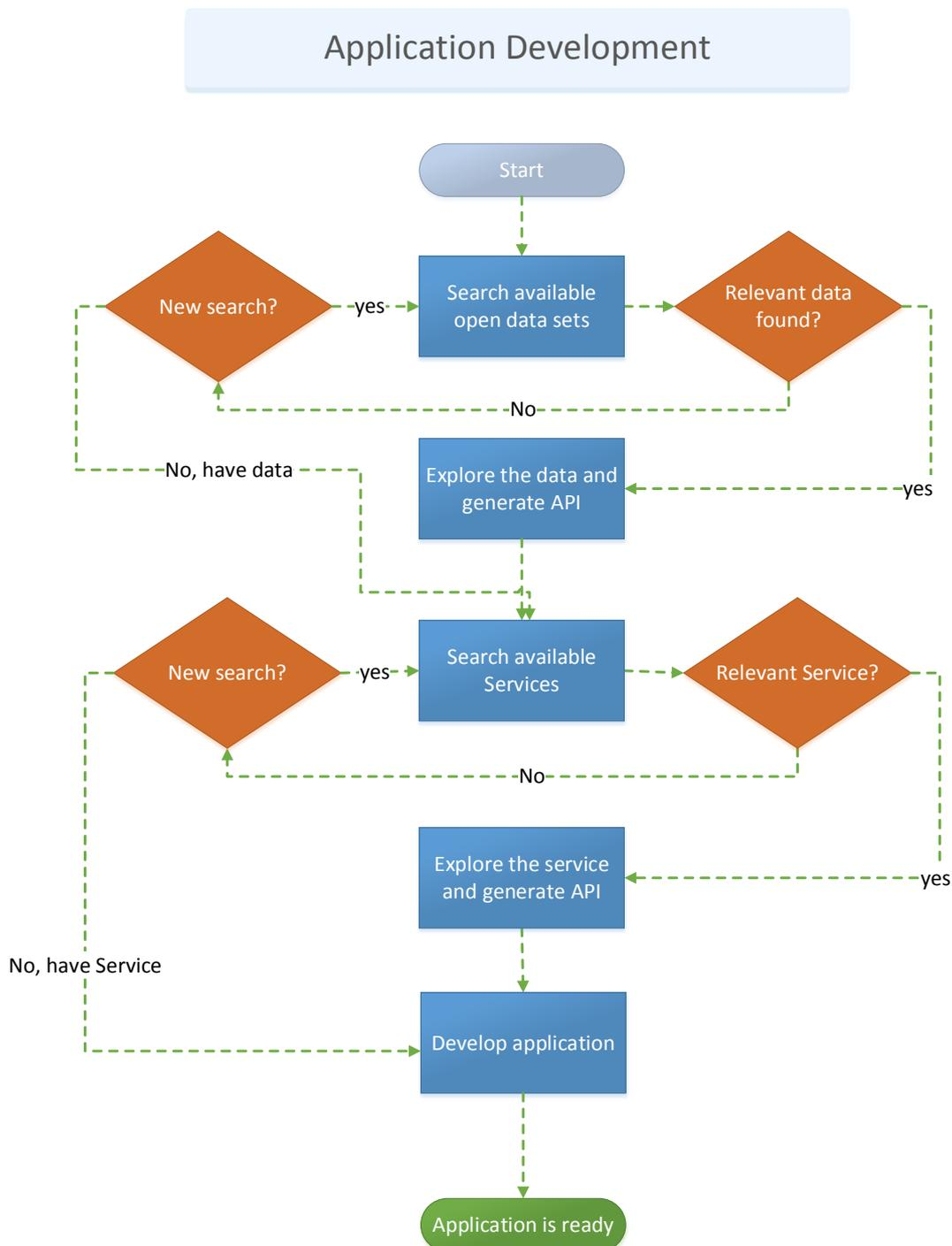
Figure 4 The SaaS components in the Workflow of the application development use-case.
